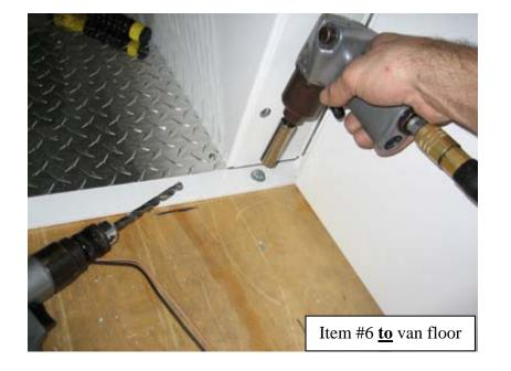
On the **Rear doorframe**, remove the sheet metal screws installed earlier. Drill 3/8" holes through the doorframe, floor, and vehicle. Attach using 3/8" x 2" hex head bolts, washers, fender washers, lock washers, and hex nuts.
